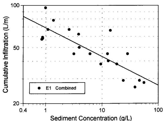
Figure 3—Cumulative infiltration (8 h) vs. average sediment concentration (initial hour) for experiment 1 and the best fit regression line. Data include combined (undifferentiated) experiment 1 data plus additional data collected from the plot during preliminary trial runs in which a range of treatments were tested.
