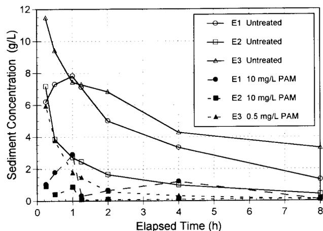
Figure 1—Sediment concentration variation over time in the recirculating furrow infiltrometer. Points represent the average for all tests for each experiment (E1-E3).
