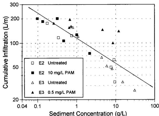
Figure 2—Cumulative infiltration (8 h) vs. average sediment concentration (initial hour) for experiments 2 (18 L/min flow rate) and 3 (23 L/min), differentiated by treatment. The best fit regression line is for the combined data.
