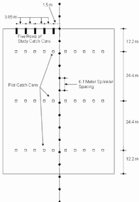
Figure 4. Plan view of line-source experimental set up (not to scale).
