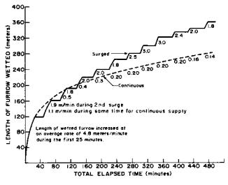
Fig. 5—Wetted front advance rates for continuous supply and surged supply which was interrupted for half of each 40-min cycle. Furrows were in a sandy loam soil near Howell, UT (Bishop et al., 1981).
