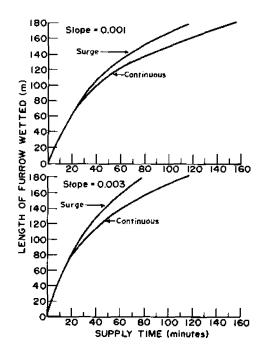
Fig. 7—Lenth of furrow wetted as a function of supply time when low stope furrows in Portneuf silt loam were provided with continuous and surged (20 min on, 20 min off) supply at the rate of 38 L/min.
