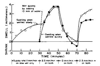
Fig. 1—Swelling and shrinkage of Portneuf silt learn soil columns on which the indicated supply rates were maintained following slow and quick wetting (adapted from Figs. 7 and 8 of Bulkock et al., 1988).
