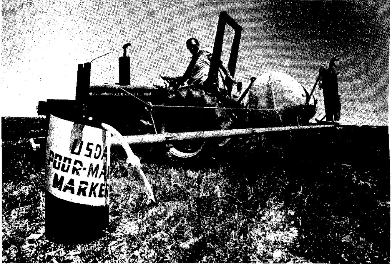
*Close-up of the marker releasing another blob of foam. Note the tractor operator pulling the string.*
