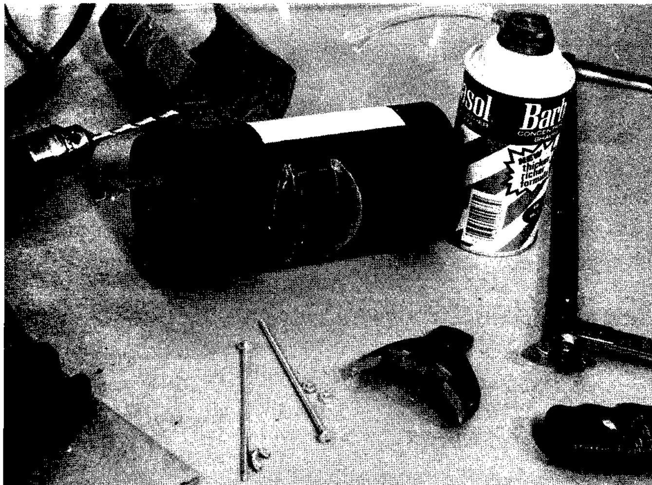
in the field, these cap-tubing units can be snapped off the empty cans and used on full ones.
