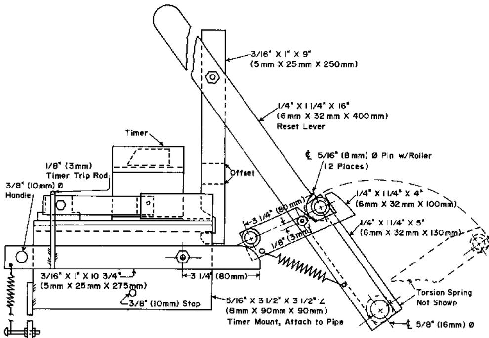
FIG. 5 Modified trip linkage for safe use of torsion spring-operated valve.
