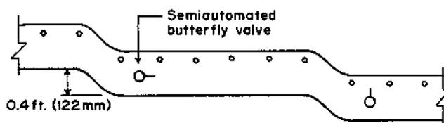
FIG. 1 Schematic diagram of semiautomated "flow-thru" gated pipe irrigation system.
