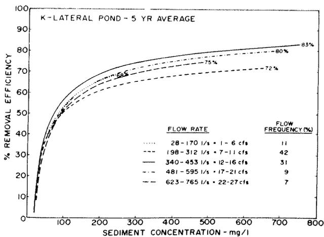
FIG. 3 The effect of sediment concentration and flow rate on the sediment removal efficiency.
