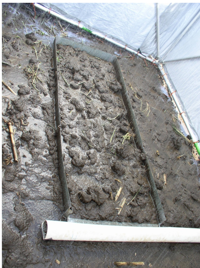
Fig. 2. Field runoff plot boundaries with runoff collection tube.
