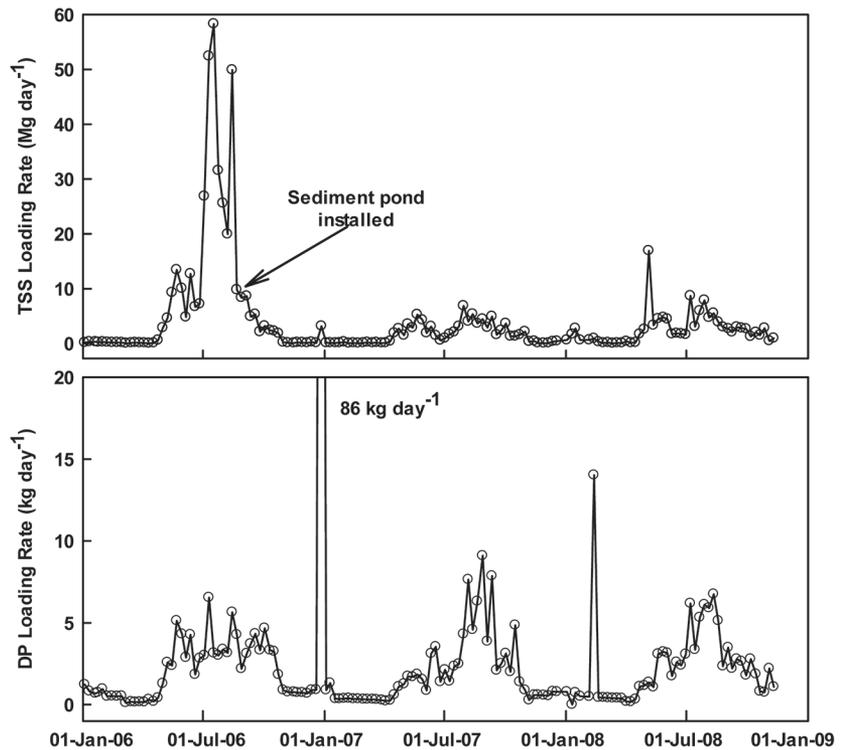
Fig. 3. Total suspended sediment (TSS) and dissolved phosphorus (DP) loading rates at a return flow monitoring site 150 m downstream from the S Coulee ponds.
