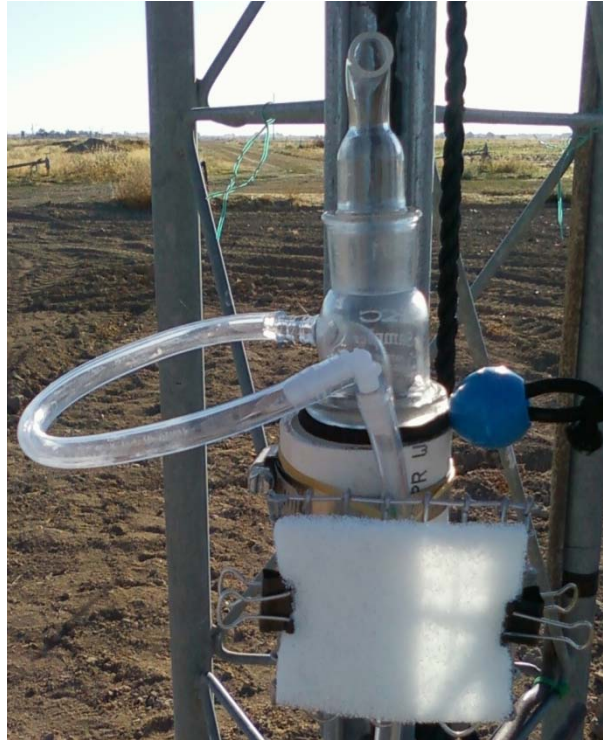
Figure 1. Impinger and passive sampler installed on the tower.
