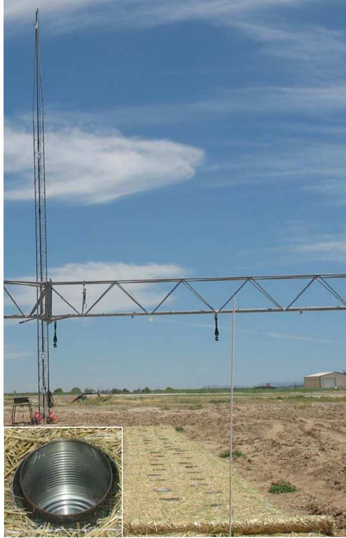
Figure 3. Test site showing layout of collectors relative to sprinkler boom and vertical sampling tower with inset close up view of collector in pit.
