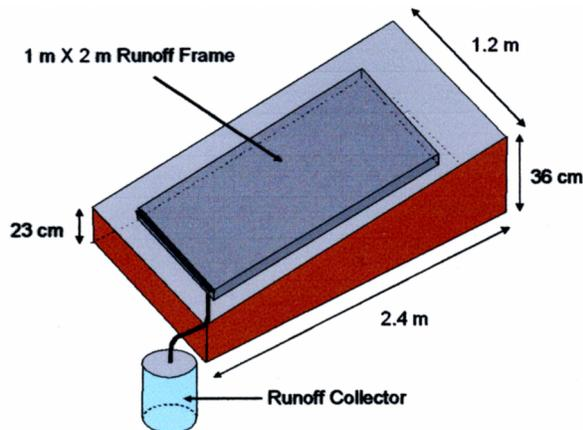
Figure 1. Diagram showing layout, dimensions, and features of elevated soil box with metal frame used for runoff plots in 2008 and 2009 runoff tests.
