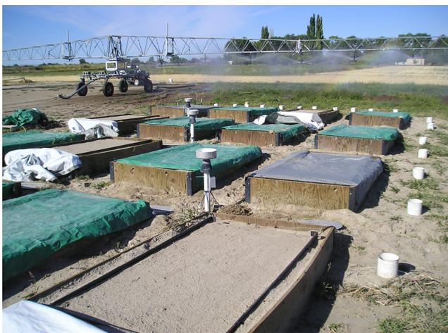
Figure 3. Experimental setup for sprinkler runoff and erosion tests in 2008 and 2009.
