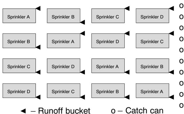
Figure 2. Diagram showing experimental design, runoff plot layout, and instrument measurement locations.
