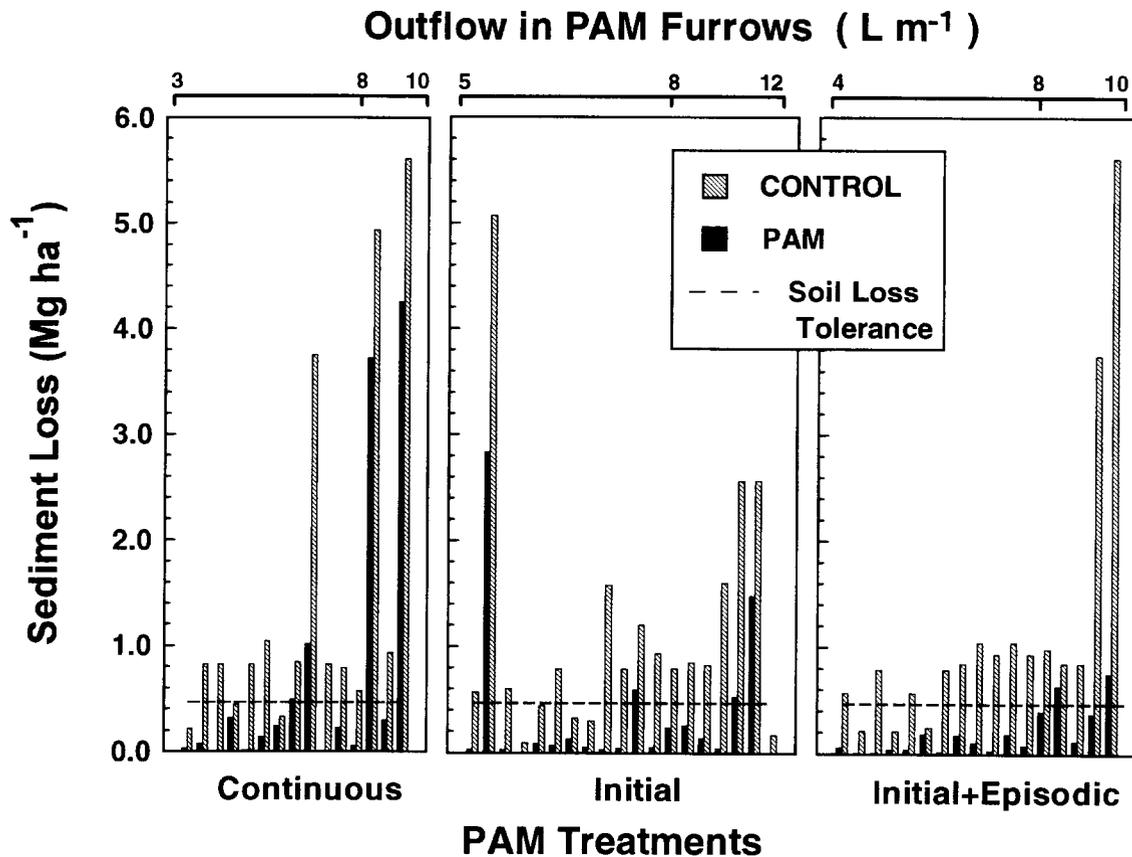
**Figure 2—Total sediment loss from individual PAM-Control comparisons (including control and PAM-treated furrows) shown for three application-strategy categories and arranged in order of increasing mean outflow in PAM-treated furrows. Pairs result from treated irrigations on freshly cultivated furrows. Within pairs, parameters were identical, but PAM application strategy, irrigation duration, inflow rates, and furrow slope varied between pairs.**
