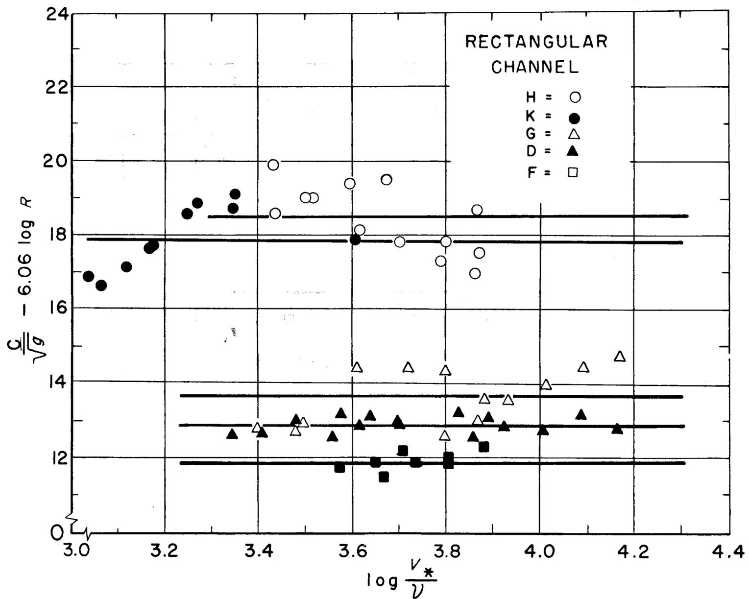
FIGURE 22.— $C/\sqrt{g} - 6.06 \log R$  as a function of  $\log V_*/\nu$  for rectangular channels. Horizontal lines represent hydraulically rough boundaries.
