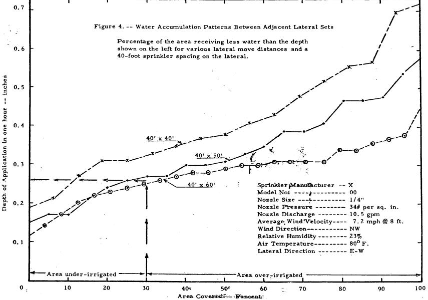
The water application efficiency obtained by the above calculation can be adjusted for wide differences in humidity, wind velocity, and temperature between the place where the sprinklers were pattern-tested and the design area by using a method such as the Frost-Schwalen nomograph.
