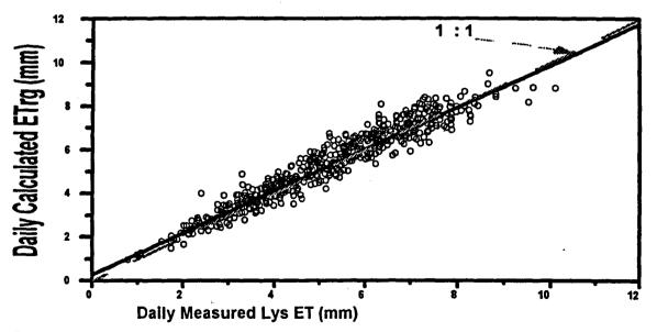
Figure 5. Comparison of grass reference ET, calculated with the modified Penman equation using a grass wind function, with lysimetrically measured fescue, reference grass ET.
