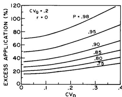
Figure 3—Excess gross water application required to complete advance on varying portions of furrow sets for varying infiltration variability ( $CV_Q = 0.20$ ).
