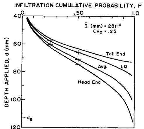
Figure 6—Distribution of water absorbed by the head end, tail end, low quarter (LQ), and whole furrow (Avg) for a rapidly decreasing infiltration relationship with the furrow-to-furrow  $CV_I = 0.25$ .
