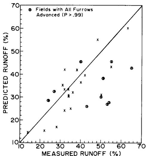
Figure 4—Runoff predicted by equation 8 vs. measured runoff from furrow-irrigated fields in southern Idaho.
