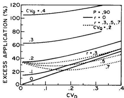
Figure 2—Excess gross water application required to complete advance on 90% of a set of furrows for varying levels of inflow and infiltration variabilities and correlation between inflow and infiltration.
