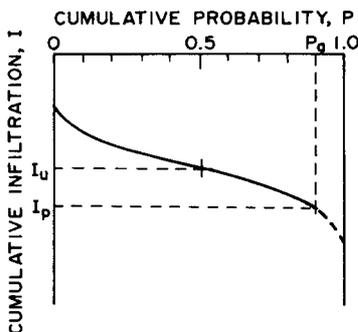
Figure 1—Typical cumulative distribution of furrow infiltration ( $CV_1 = 0.25$ ).
