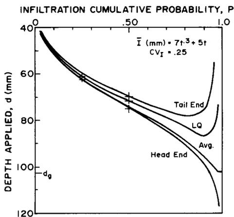
Figure 7—Distribution of water absorbed by the head end, tail end, low quarter (LQ), and whole furrow (avg) for a relatively constant infiltration relationship with the furrow-to-furrow  $CV_I = 0.25$ .
